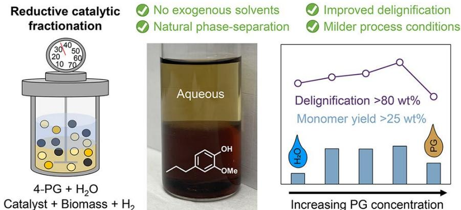
Process schematic highlighting biphasic solvent behavior and promising RCF performance of 4-propylguaiacol/water mixtures
