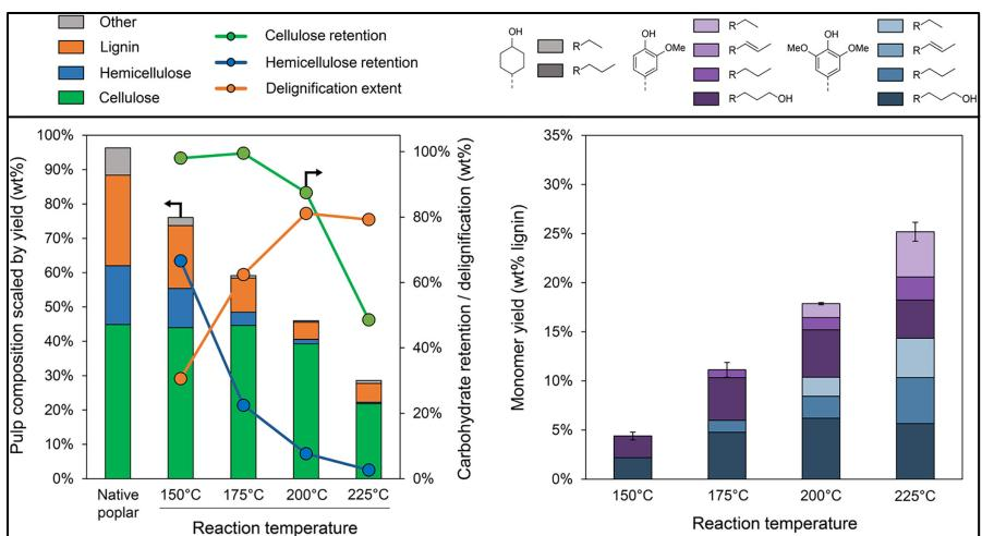
Plots highlighting the inherent tradeoff between lignin extraction and depolymerization and varying reaction temperatures
