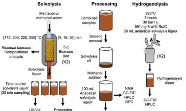
Left: Approach to evaluate lignin condensation rates and delignification extents in a flowthrough reactor.
