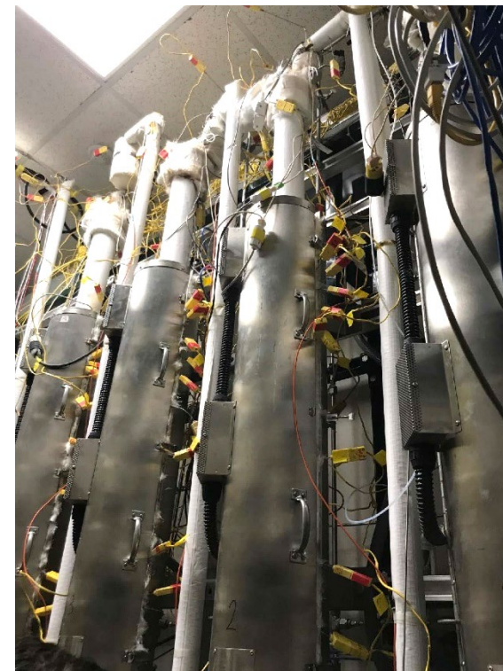
Vertimass LLC's demonstration reactor for single-step ethanol conversion. Credit: Vertimass
