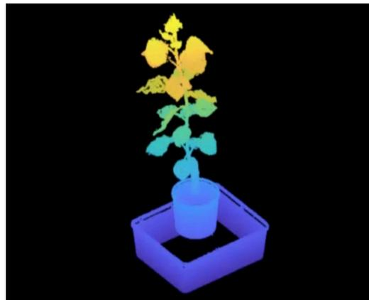
The Advanced Plant Phenotyping Laboratory will gather multiple plant phenotypes at high throughput generating terabytes of data. (Top) The poplar plants are grown on a conveyor belt in a greenhouse and sent for regular automated imaging. (Center) Hyper-spectral images indicate leaf water, nitrogen, and biochemistry. (Bottom) A computer reconstruction of the plant. [Courtesy CBI]
