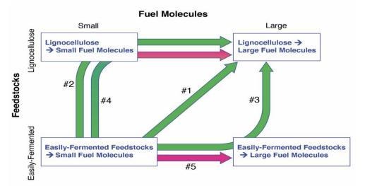
Alternative research and commercialization paths. Biological conversion. Catalytic conversion. #4 is the only path leading to cellulosic biofuels that does not require biological production of large fuel molecules.
