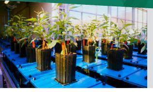
ORNL's plant phenotyping system aids scientists in connecting plant gene functions to observable traits through automated, highthroughput measurement of key plant characteristics.
