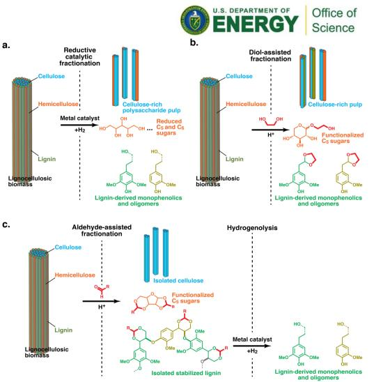
Three lignin-first strategies using solvolysis and catalytic stabilization of reactive intermediates to stable products or protection-group chemistry and subsequent depolymerization
