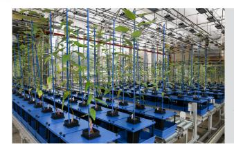
ORNL's plant phenotyping system aids scientists in connecting plant gene functions to observable traits through automated, high-throughput measurement of key plant characteristics.
